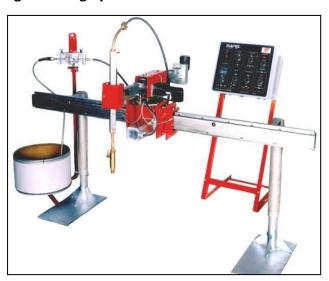
This VOW45 was built with a set of fixtures and a chuck drive system for turn rolls and welding using a manual sub arc process. The open carriages were used to keep the system back for the work zone to minimize heat induced in the drive motors.
