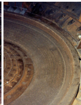
Segmented Grinding Ring: After Hardfacing
