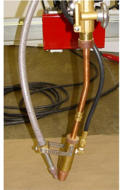
The drawing below shows a typical torch assembly. The radius of the bend and resulting angle can all be customized to fit your welding application. This design includes a 6" extension to reduce cost when replacement parts are required.
