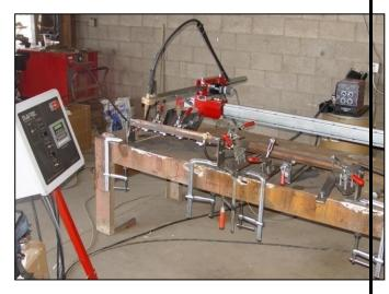
The machine to the right was a dual torch welding system for hardfacing the OD of the part. Mavrix manufactured this system including the turning rolls.
