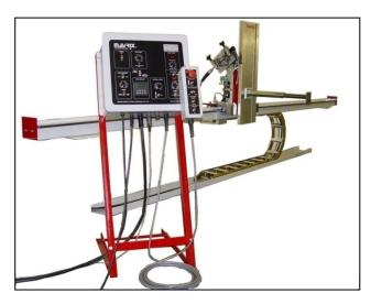
The system to the right was built complete by Mavrix. It included the headstock, tailstock, pre-heat burners, and angular axis adjustment and in the final configuration included a water cooled torch.
