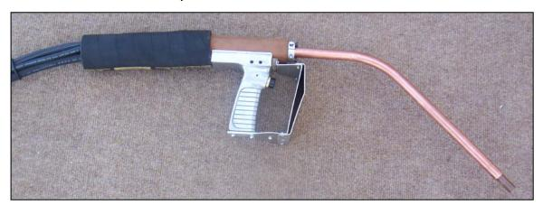
This gun assembly uses an electric push button trigger which requires little pressure to actuate. An alternate trigger circuit is available on the PA-10 that when used with this gun allows the operator a single touch of the trigger to start welding and a single touch to stop. Assembled ready to plug into the Mavrix PA-10 wire feeder and supplied with a lug for quick termination.
