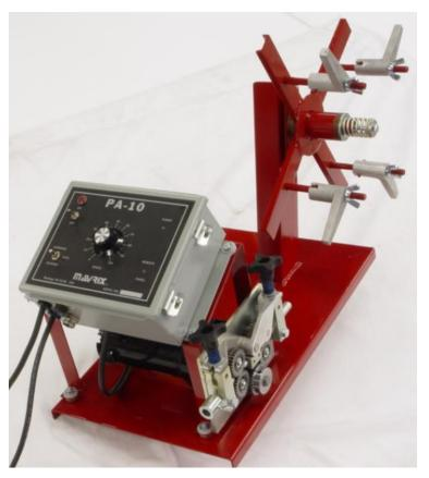
The wire feeder to the right is shown with the optional gas solenoid and a post mounting. This unit is intended to plug directly into a Mavrix control.
