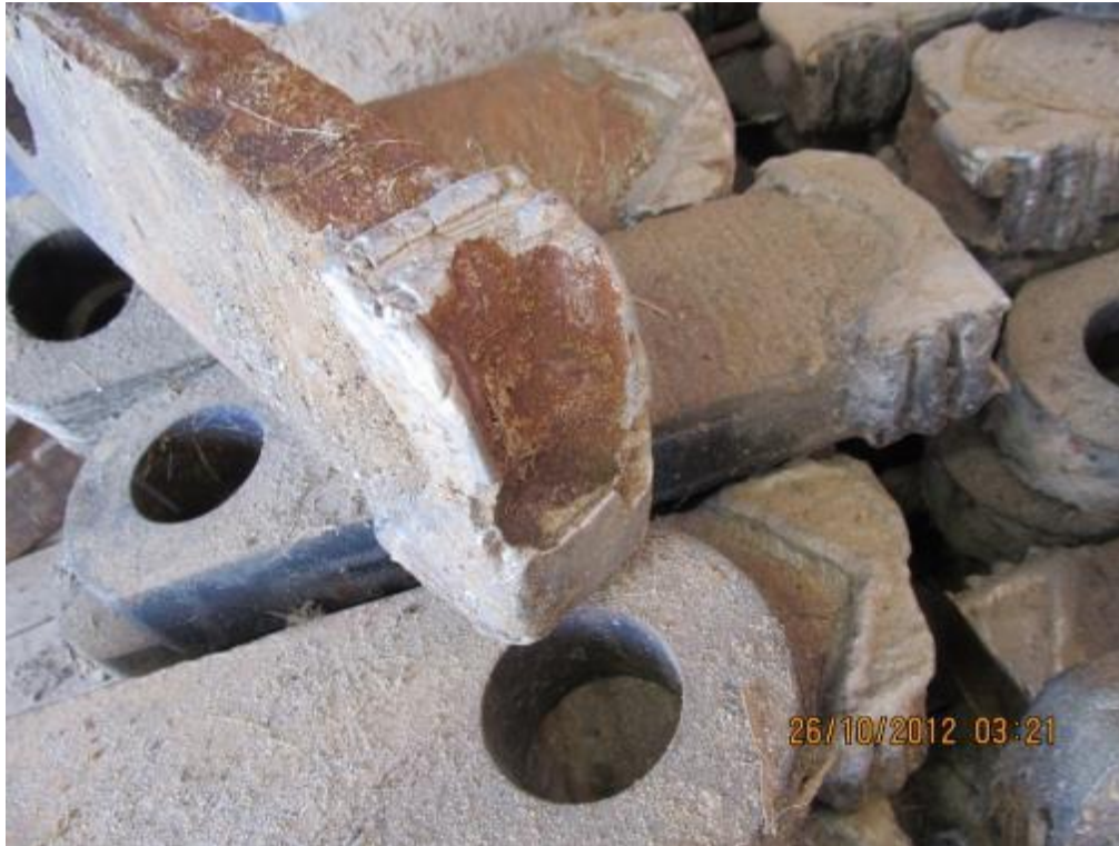
Wear pattern from impact and abrasion
